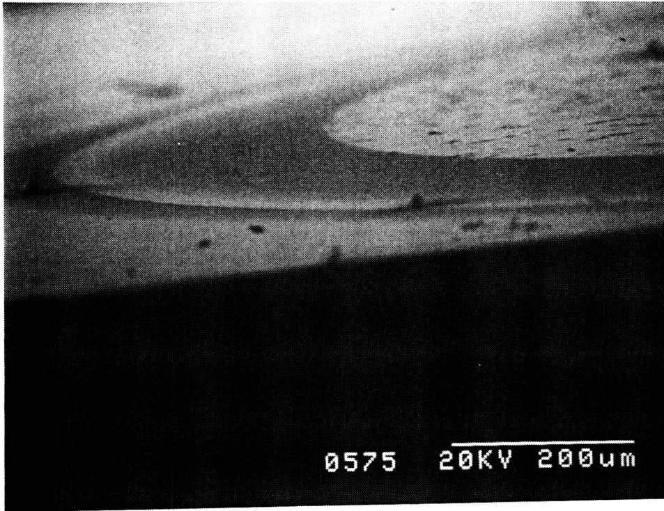
Fig. 5 SEM of shoulders left when tool is lifted suddenly during facing cut. In the sample above, the tool was lifted suddenly and allowed to continue the facing for a short distance.
