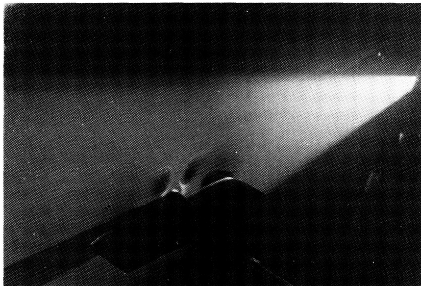
Figure 51. Laser vapor screen photograph as observed from a three-quarter left rear view. M_{\infty} = 1.10 , \alpha = 20^{\circ} .
