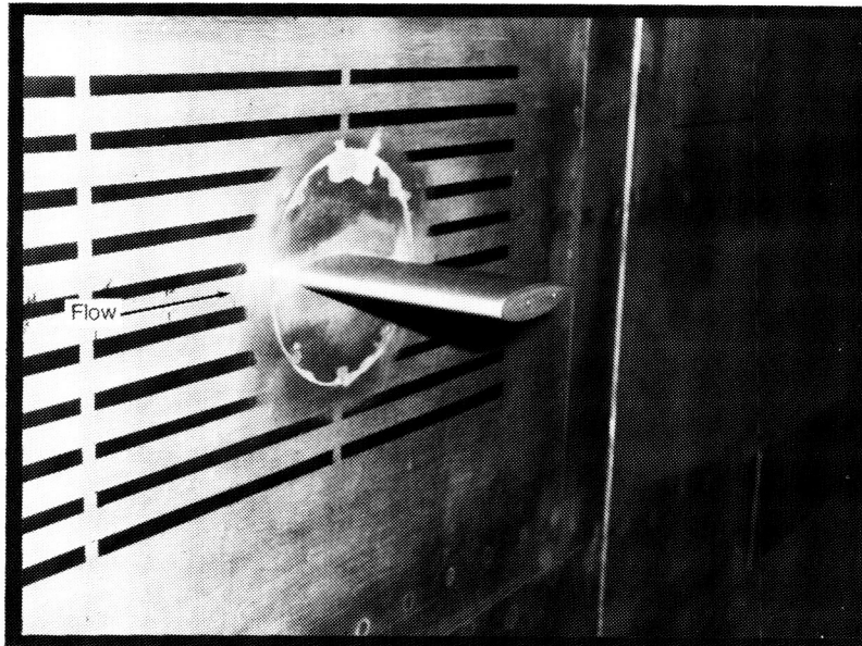
Figure 15. Airfoil mounted on the sidewall of the NTF for tests of the hot-film dielectric.
