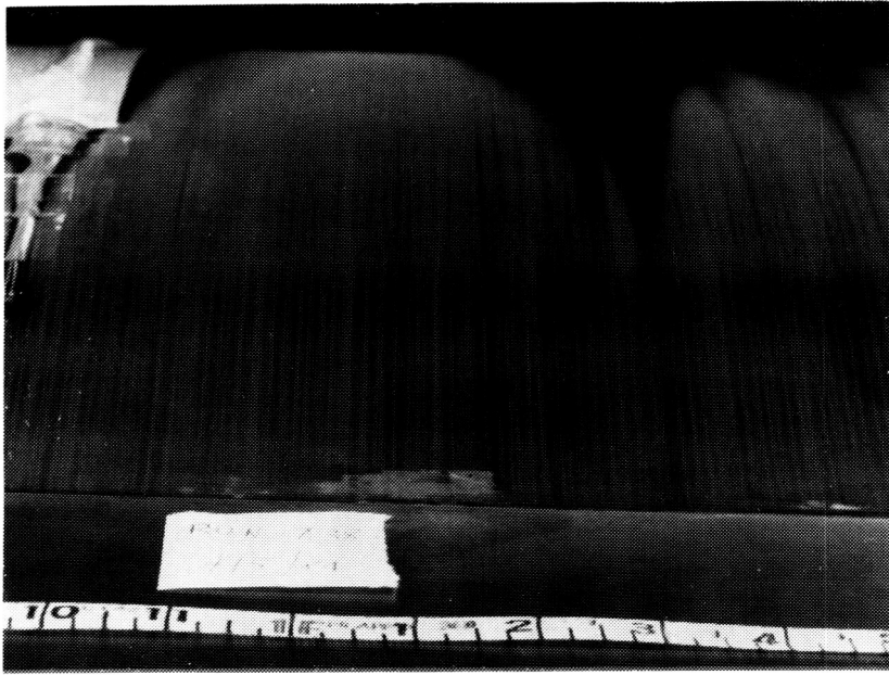
Figure 40. Flow-visualization picture of Taylor-Gortler vortices in airfoil concave region looking downstream.
