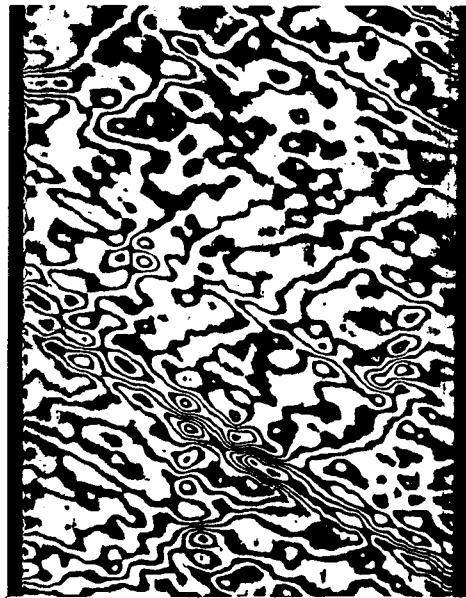
Fig. 1. Photograph of a moire interferometric fringe pattern that provides a full-field map of the in-plane axial displacement. The pitch of the reference grating has been adjusted to subtract out the uniform axial tensile elongation leaving only the nonuniform portion. (Courtesy of the VPISU Photomechanics Laboratory; D. Post, Director)
