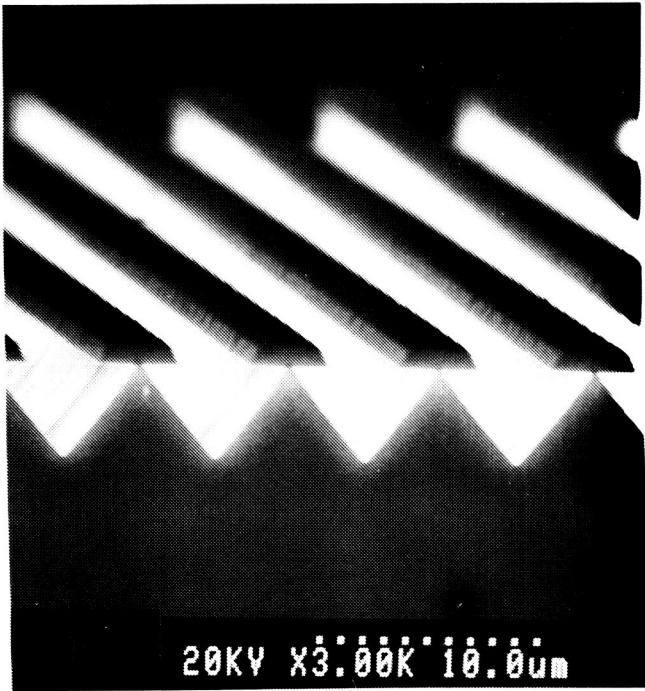
FIGURE 3. - MICROGRAPH AFTER 150s ETCH IN CAROS ETCHANT AT 24 °C.
