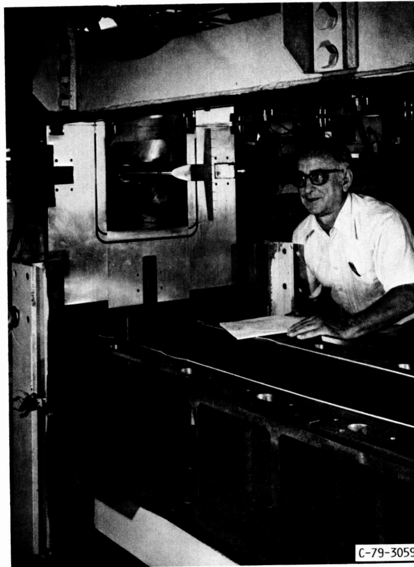
FIGURE 3. - 1 FT BY 1 FT SUPERSONIC WIND TUNNEL TEST SECTION.
