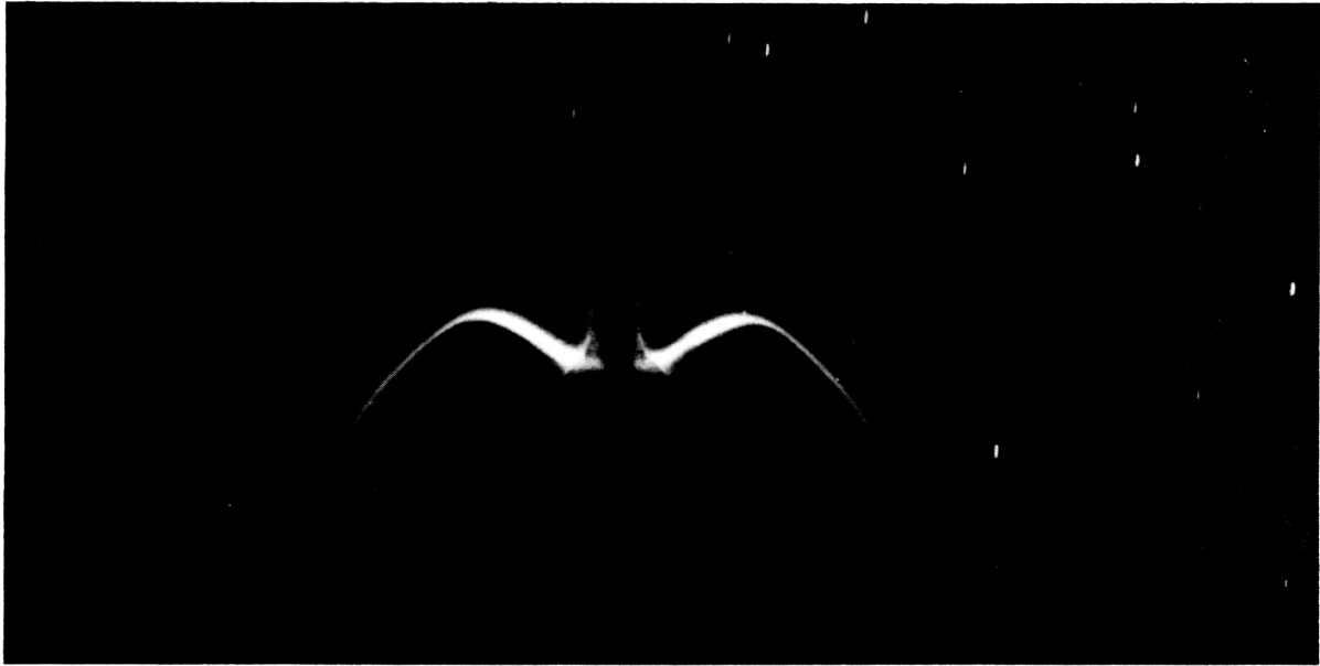
Figure 9.- Glow photograph of the Orbiter, the OMS pods, and the vertical stabilizer during the STS-8 mission. The orange glow appears above the OMS pods, which are in ram. Note that the stars are streaked in the direction of the velocity vector.
