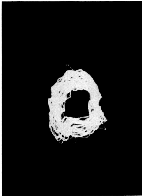
Fig. 6 - b Fig. 6 Orbit of shaft centre a - normal state b - transient state c - unstable state
