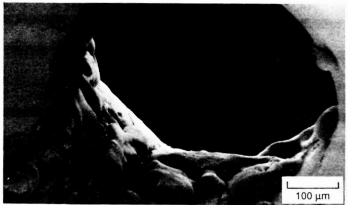
(c) SEM of constrictor (post test).
