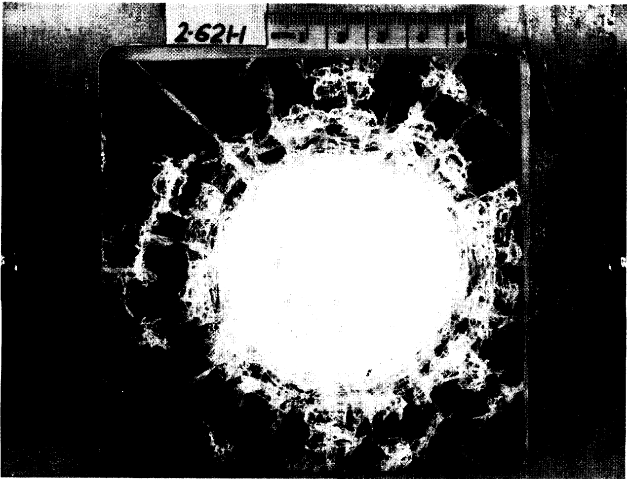
Damage to a 2 cm thick Glass Target by a 0.15 cm Projectile at 7.3 km/sec.
