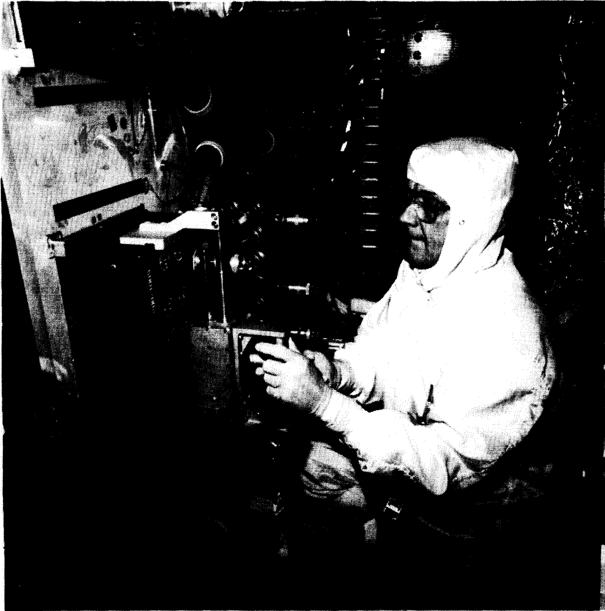
Figure 6. Fit checks with early prototype handhold verified acceptability of envelope and mission suitability. Astronaut Bruce McCandless performs the test.
