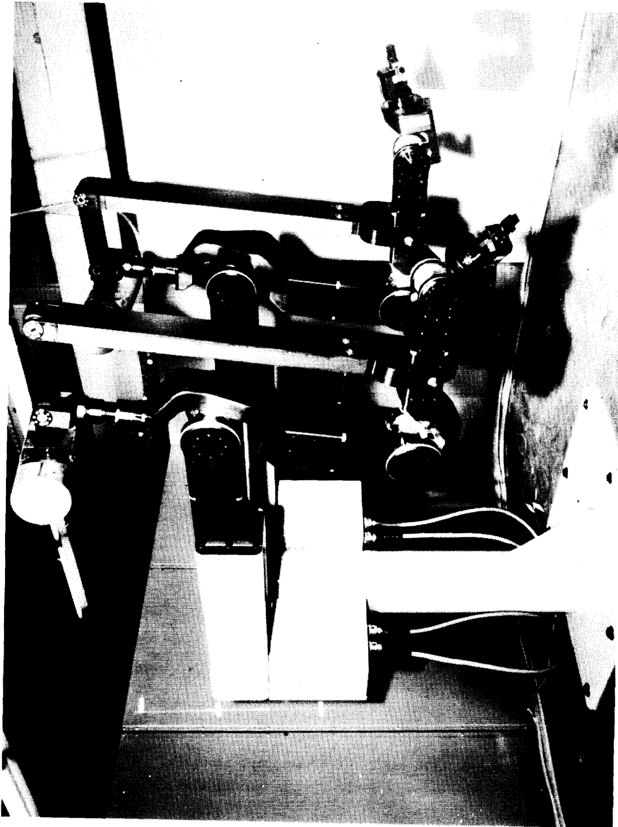
Figure 1. Laboratory Telerobotic Manipulator (LTM) slave.
