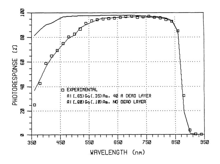
Figure 6. Experimental Data and Calculated Values for Internal Photoresponse Assuming x = 0.9 and No Dead Layer, and x = 0.65 and a Dead Layer Thickness of 40 A.
