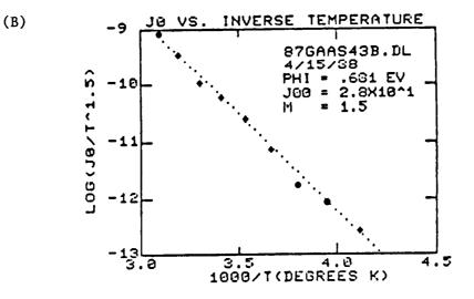
Figure 12. J -T Analysis for GaAs Cell 87-43. (A) Log J versus T<sup>-1</sup> for the Large Voltage Mechanism. (B) Log J versus T<sup>-1</sup> for the Low Voltage Mechanism.
