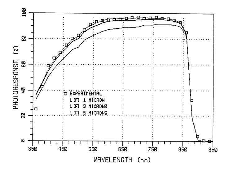
Figure 7. Calculated Values of Internal Photoresponse for a Range of Values for the Emitter Diffusion Length, L(F).
