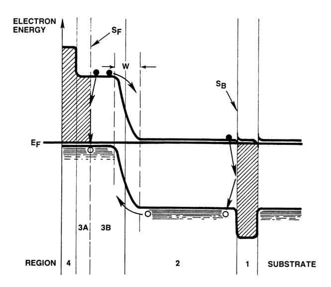
Figure 3. Assumed Electron Band Structure for GaAs Cells.
