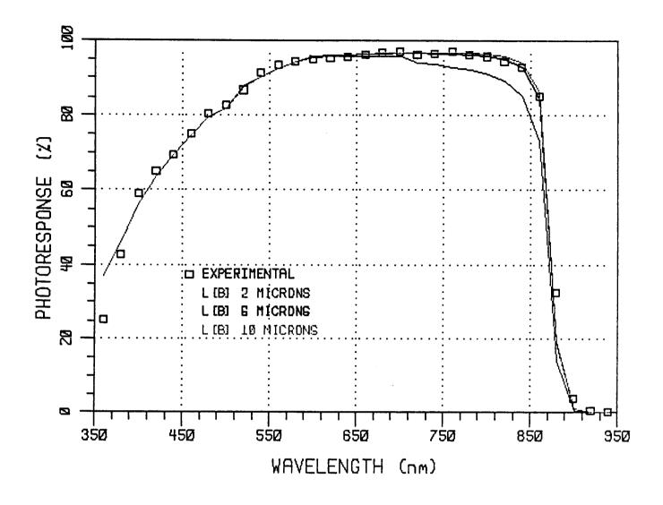
Figure 9. Calculated Values of Internal Photoresponse for a Range of Values for the Base Diffusion Length, L(B).
