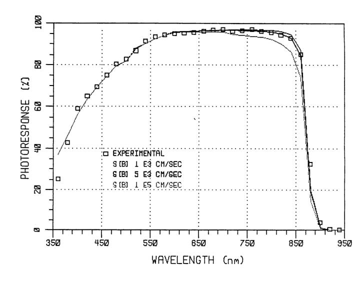
Figure 10. Calculated Values of Internal Photoresponse for a Range of Values for the Surface Recombination Velocity at the Back Surface, S(B).
