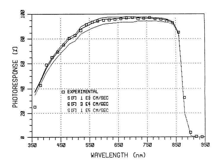
Figure 8. Calculated Values of Internal Photoresponse for a Range of Values for the Emitter Surface Recombination Velocity, S(F).
