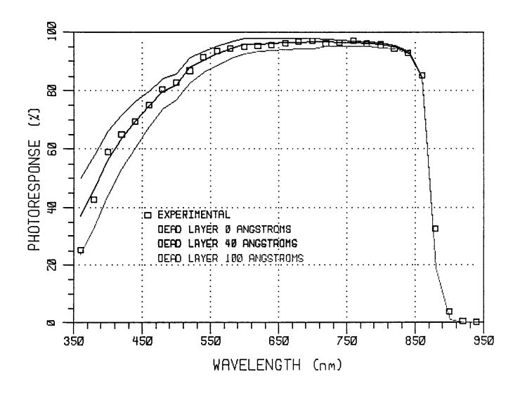
Figure 5. Experimental Data and Calculated Values for Internal Photoresponse versus Wavelength for Three Dead Layer Thicknesses.
