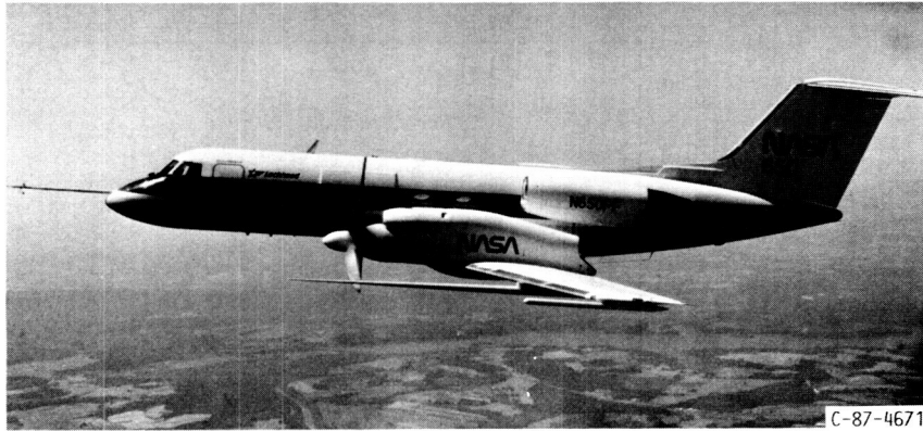
(a) NASA PTA INSTALLED ON LOCKHEED G11 AIRCRAFT.
