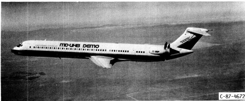
(c) NASA/GE UDF INSTALLED ON MCDONNELL DOUGLAS MD-80 AIRCRAFT.
