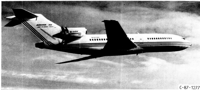
(b) NASA/GE UDF INSTALLED ON BOEING 727 AIRCRAFT.
