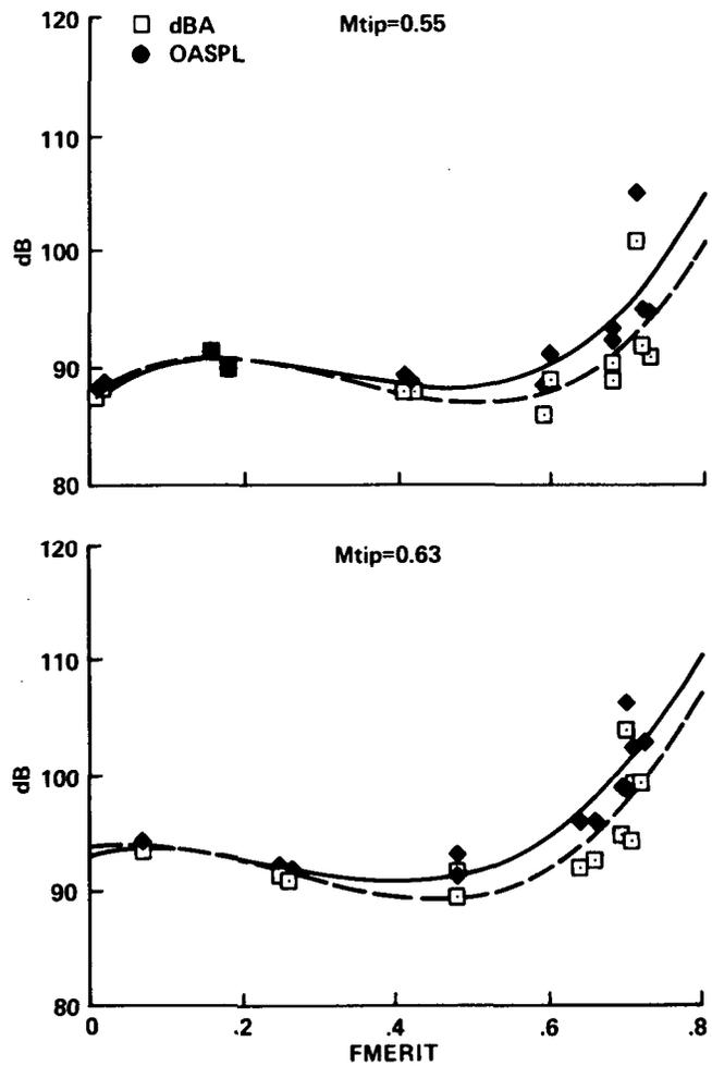
Figure B11.— Acoustic levels as a function of FMERIT at two values of  $M_{tip}$ . Microphone No. 8:
