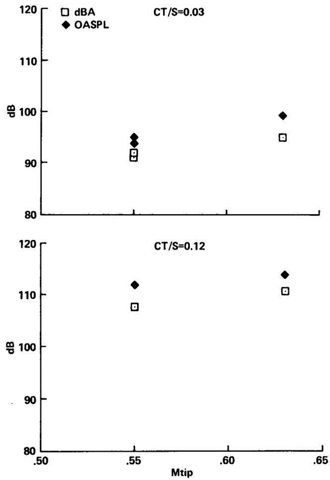
Figure B1.— Acoustic levels as a function of  $M_{tip}$ . Microphone No. 5:  $r/D = 1.0$ ,  $\psi = 180^\circ$ ,  $\theta = +10^\circ$ .
