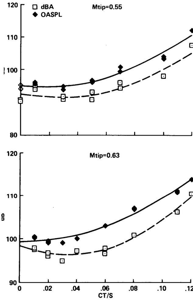
Figure B5.— Acoustic levels as a function of  $C_T/\sigma$  at two values of  $M_{tip}$ . Microphone No. 5:  $r/D = 1.0$ ,  $\psi = 180^\circ$ ,  $\theta = +10^\circ$ .
