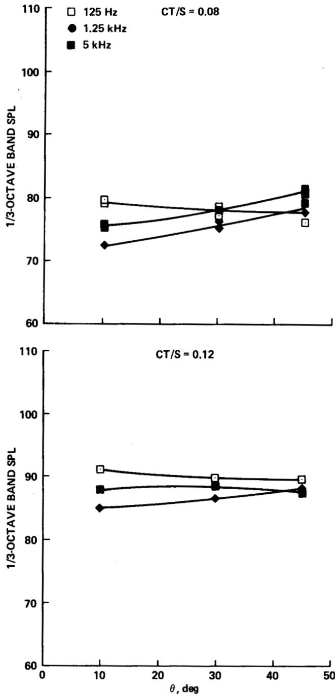
Figure C3.— Acoustic levels at four frequency bands as a function of elevation angle (directivity):
