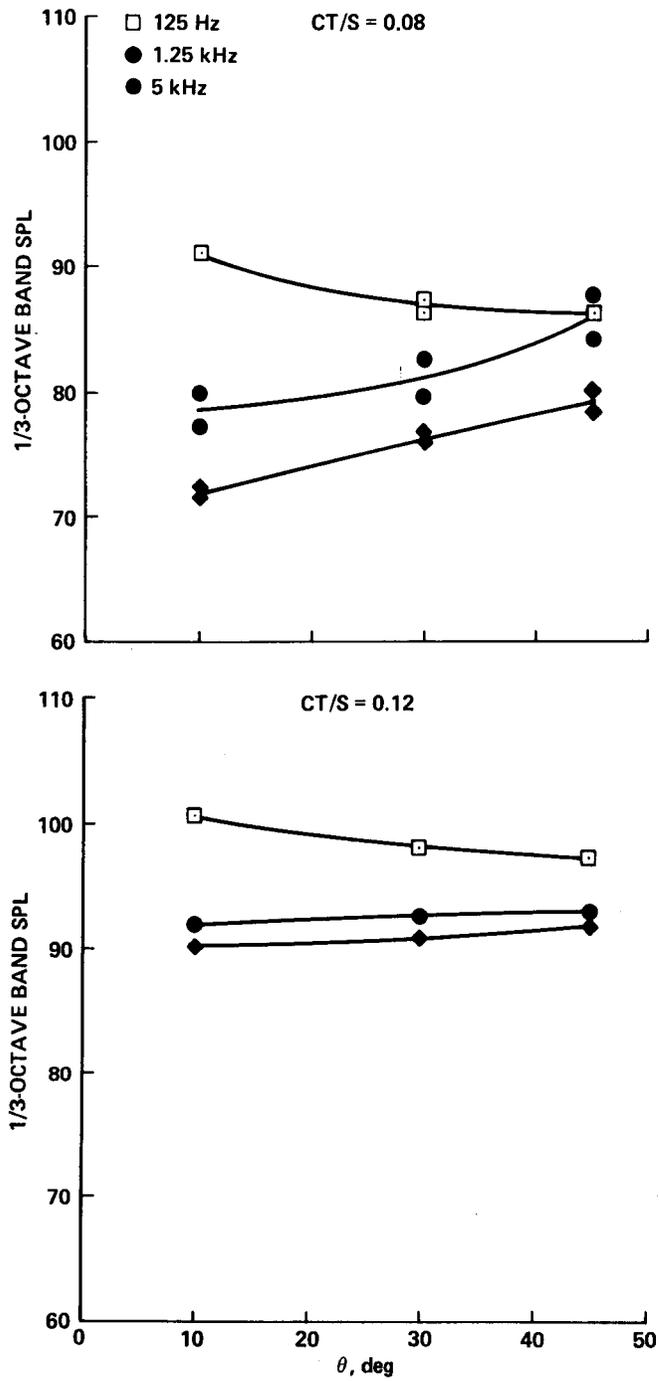
Figure C4.- Acoustic levels at four frequency bands as a function of elevation angle (directivity):
