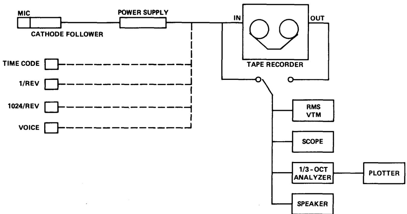
Figure 3.— Acoustic data acquisition and reduction system.
