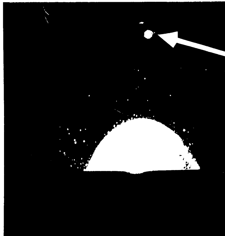
Figure 9. Ejecta splash back from a 0024 airfoil at random times after impact. Note incoming droplet in lower photograph.
