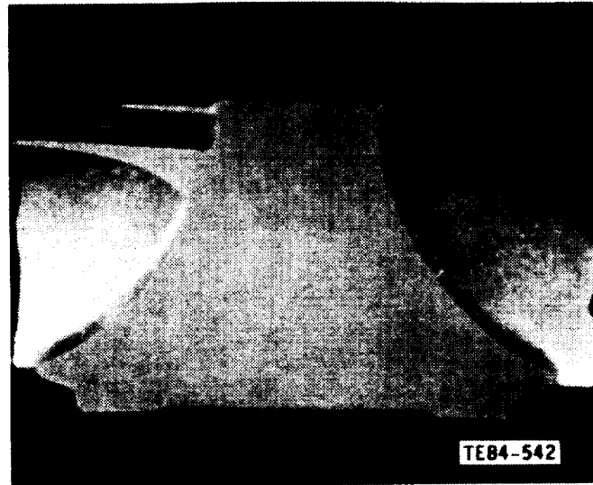
Figure 17. Internal structure of GTE injection-molded and HIP-processed AY6 \text{Si}_3\text{N}_4 rotor.
