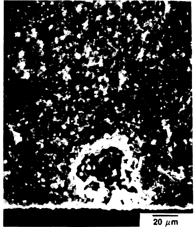
Figure 18. Typical microstructure of GTE AY6 SSN material.
