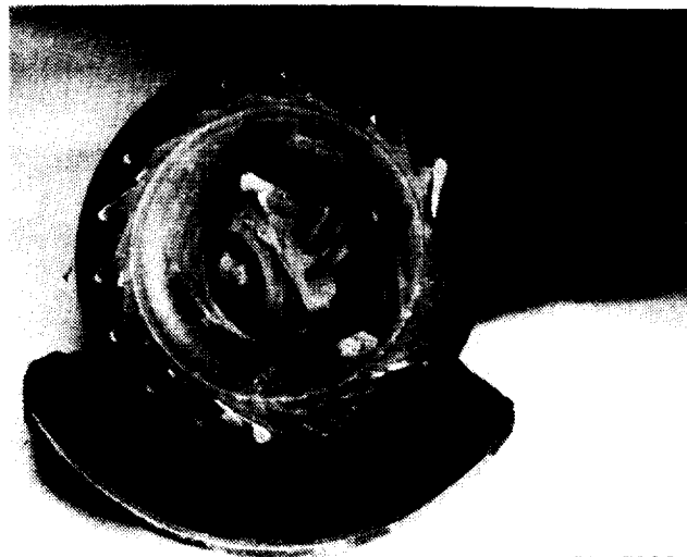
Figure 114. As-torn-down condition of the gasifier turbine rotor, which was wedged in the scroll shroud.
