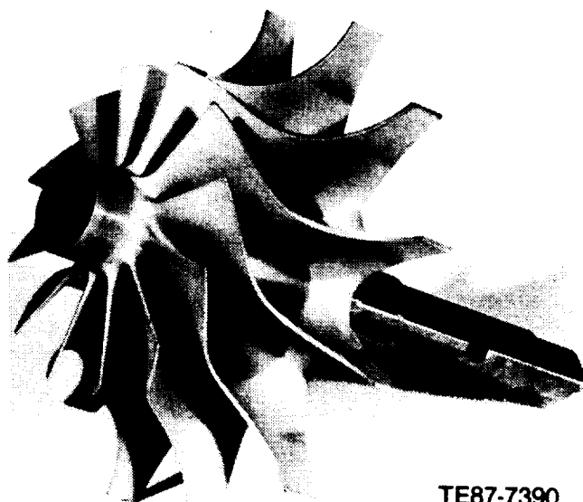
Figure 187. Power turbine rotor S/N 0002-1 prior to test.
