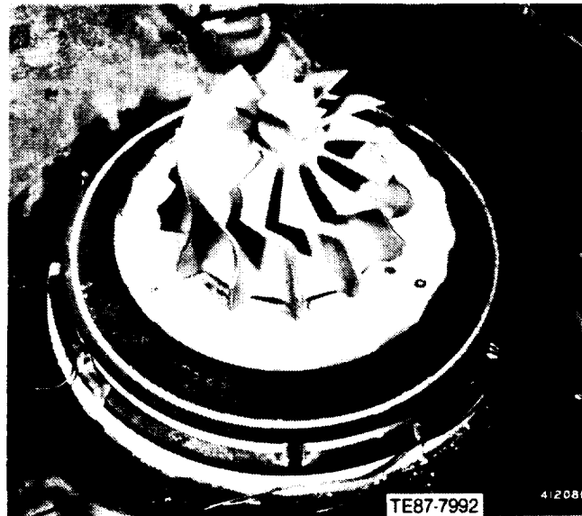
Figure 103. A Si_3N_4 gasifier turbine rotor lost all inducer tips after engine testing for 99:54 hr in engine S/N 1, BU20.
