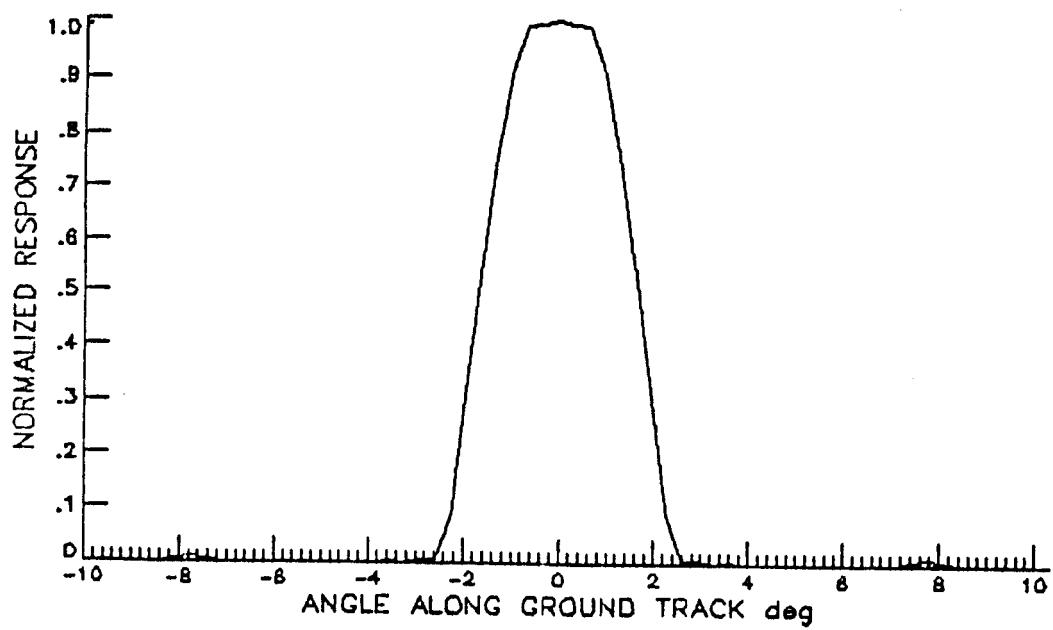
Figure A1. ERBE scanner point spread function.
