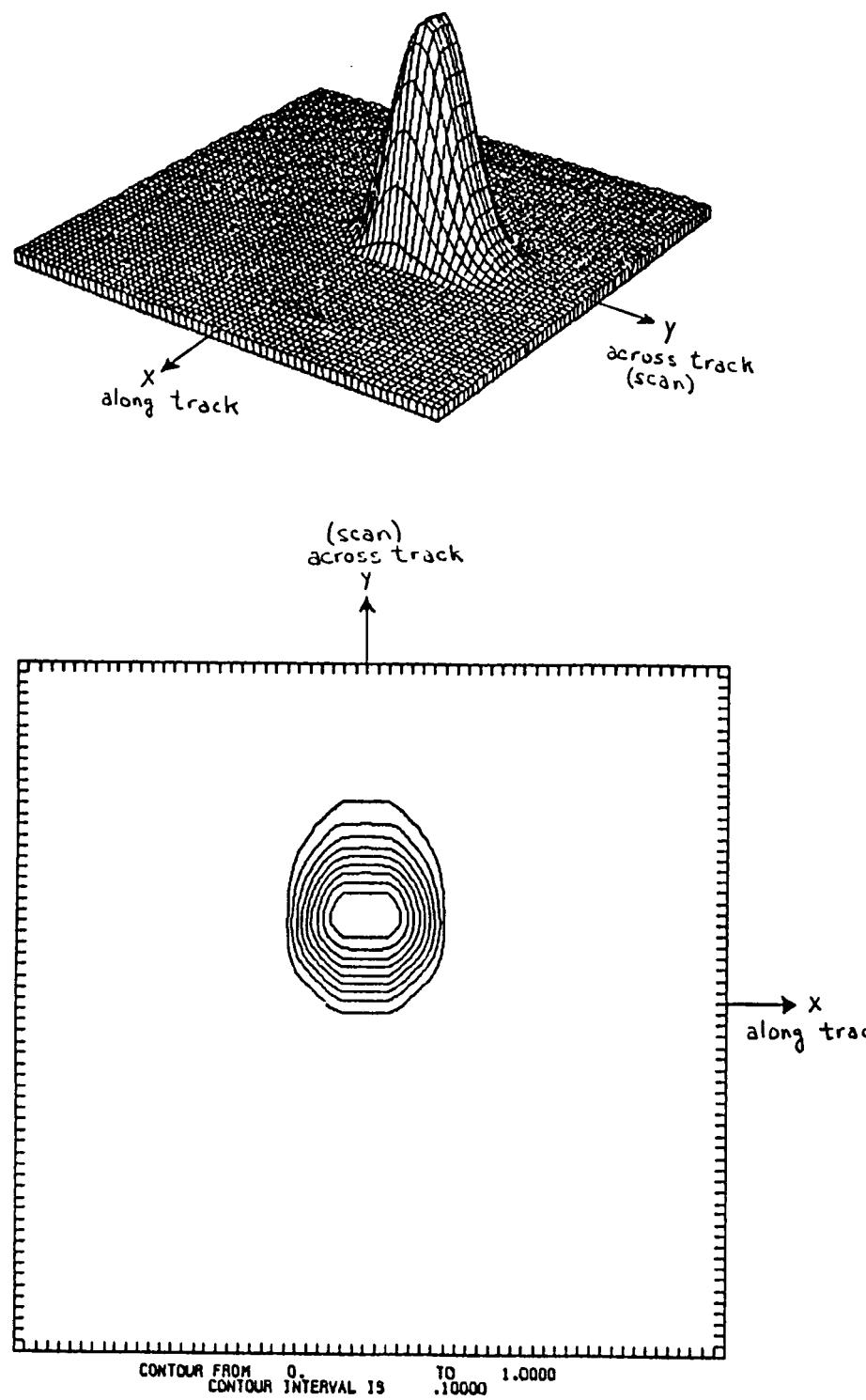
Figure A2. Additional views of ERBE scanner point spread function.
