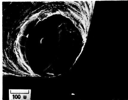
(D) SECOND TWO PERCENT THORIATED TUNGSTEN TIP AFTER TWO HOURS OF OPERATION. (150x).
