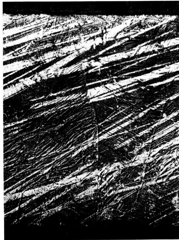
Figure 13. Micrographs of Cold Rolled Ti-6Al-4V Alloy Strip
