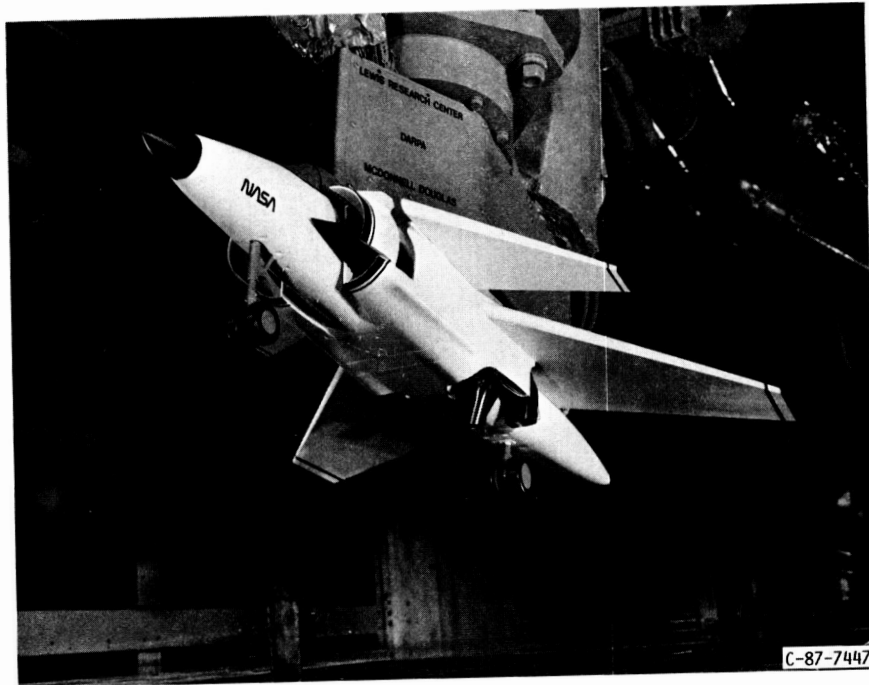
FIGURE 4. - THREE-QUARTER FRONT VIEW OF A 9.2-PERCENT-SCALED SHORT TAKEOFF AND VERTICAL LANDING (STOVL) MODEL IN THE 9- BY 15-FOOT LOW-SPEED WIND TUNNEL (LSWT).
