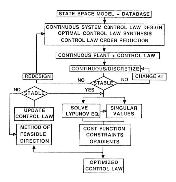
FIG. 1 Optimization scheme block diagram
