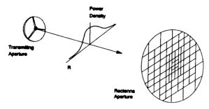
The focusing elements in the center of the rectenna array are smaller.
