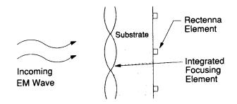
The integrated focusing element will reduce the loss to surface waves
