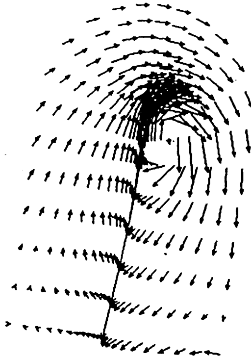
Figure 23. Secondary Flow Vectors at X/D = -0.036 , 2% Thick Blade.
