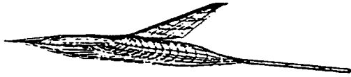
Fig. 16 Grid generated about Wing-C with an incompatible root section and fuselage cross section
