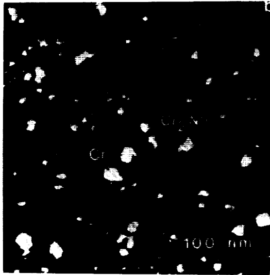
38b - Dark Field View of Figure 38a Using the First Imaging Condition. Both Cr and Cr 2 Nb Precipitates Are In Strong Contrast.
