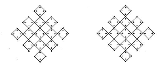
Figure 2: Two of the 1024 code words of a three-shell diamond lattice network storing the subcode  $\{(+ + ++), (+ - +-)\}$  in each of the subnetworks.
