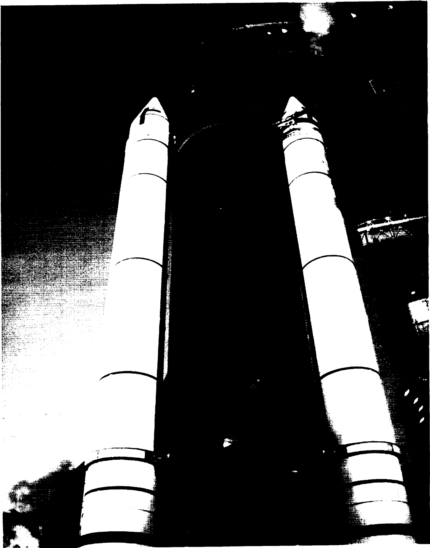
Overall view of the Solid Rocket Boosters/External Tank -Z side Note reflection of condensate on aft hardpoint TPS closeout
