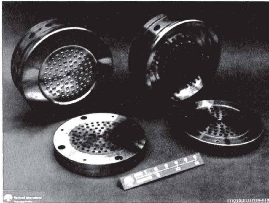
Figure 3 – Injector Assembly Details Including Injector Bodies and Faceplates
