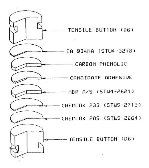
Figure 4. Tensile Button Configuration
