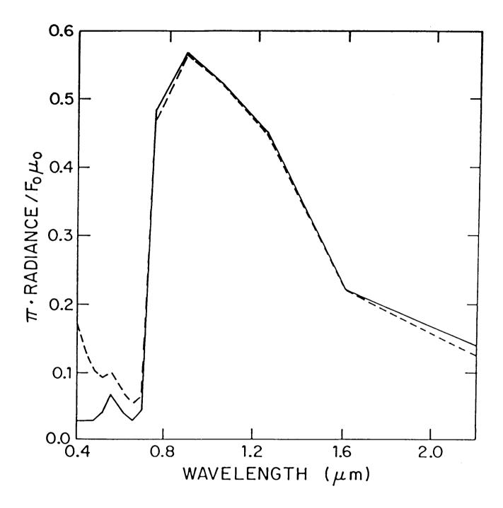
Figure 1. Surface reflectance (——) and the corresponding radiance (- - -) above the atmosphere for a typical vegetation. The radiance is normalized by  $F_0$ , the incident solar flux, and by  $\mu_0$ , the cosine of the solar zenith angle (from Kaufman, 1987).
