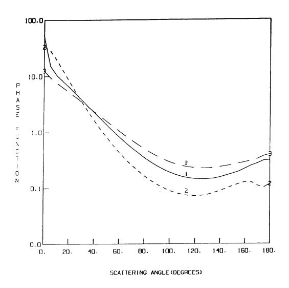
Figure 5. Aerosol single scattering phase functions derived from: 1) bimodal log-normal aerosol size distribution used in the unperturbed model (——), 2) single log-normal aerosol size distribution with an index of refraction n = 1.349 - 0.008i, geometric mean mass radius  $r_m = 0.6 \, \mu m$ , standard deviation of the logarithm of the radius  $\sigma = 0.61$  (--), and 3) power law aerosol size distribution with  $\nu = 4$  and an index of refraction  $n = 1.53 - 10^{-7}i$  (——).
