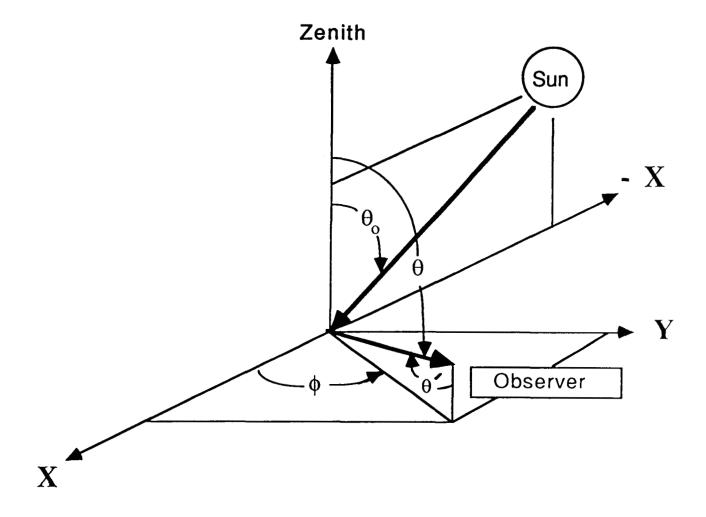
Figure 2. Angular coordinates used in the algorithm. The X-Y plane is a horizontal plane tangent to the earth's surface at the observation point. The solar zenith angle  $\theta_0$ , observation zenith angle  $\theta$ , observation scan angle  $\theta$ ', and observation azimuth angle  $\phi$  are shown. In this particular representation of planar geometry  $\theta = \theta$ '; the general relationship is given by eq. (9).
