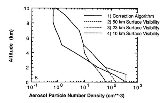
Figure 4. Aerosol particle number density profiles for: 1) 'average' distribution of Braslau and Dave (1973) used in the correction algorithm; 2) 50 km surface visibility, 3) 23 km surface visibility, and 4) 10 km surface visibility models from Shettle and Fenn (1979). Figure 4a is for altitudes between 10 and 70 km while figure 4b is for altitudes between 0 and 10 km. These profiles have been normalized for an aerosol optical thickness  $\tau_a = 0.25$  at 0.55  $\mu$ m.
