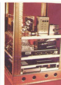
This apparatus was flown on the Lear jet to produce the polymer composites.
