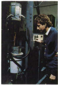
The center's Low-voltage Scanning Electron Microscope is used to examine metals, ceramics, polymers, and composite materials directly without the application of coatings and is particularly useful for viewing fractured or damaged surfaces.
