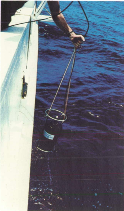
Biospherical Instruments, Inc.'s sensors, which measure ambient light below the ocean's surface, are shown being lowered into South Pacific waters from the Calypso. The instrument was tested during a cruise sponsored by the Cousteau Society.
