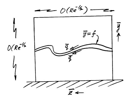
Figure 1 (b) Cross-section  $O(Re^{-\frac{1}{2}} \times Re^{-\frac{1}{2}})$  in the vortex/Rayleigh-wave case of Sections 4, 5, including the critical-layer  $O(Re^{-\frac{2}{3}})$  thick) effect at  $\overline{y} = f$ .
