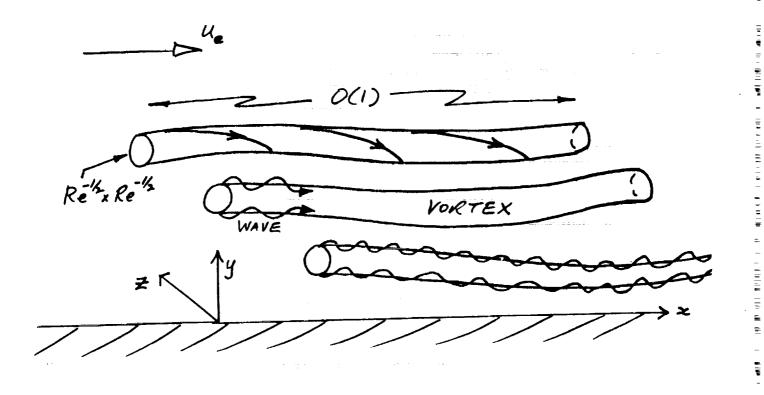
Figure 1 (a) Typical strongly nonlinear vortex/wave interactions in a boundary layer.
