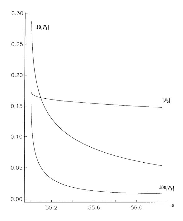
Figure 3(b) The development of  $P_0, P_1, P_2$  with x for the case  $\Delta = .02, P_0 + \sum_{1}^{infty} P_n = .2$  at  $\bar{x} = 55$ .
