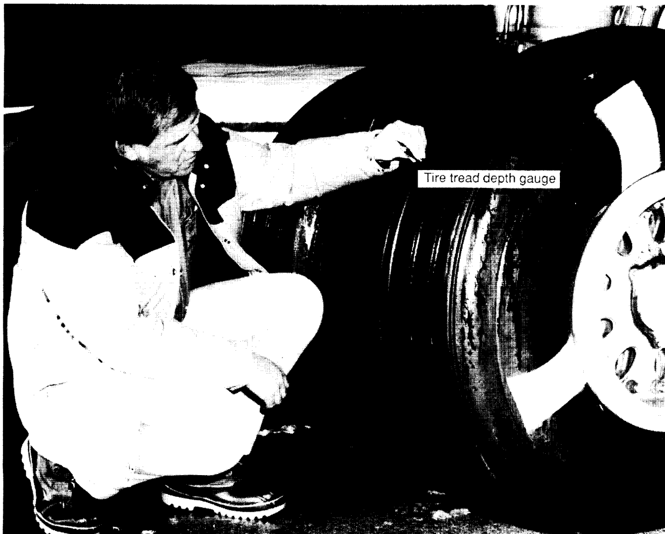
Figure 41. Measurement of aircraft tire tread groove depth.
