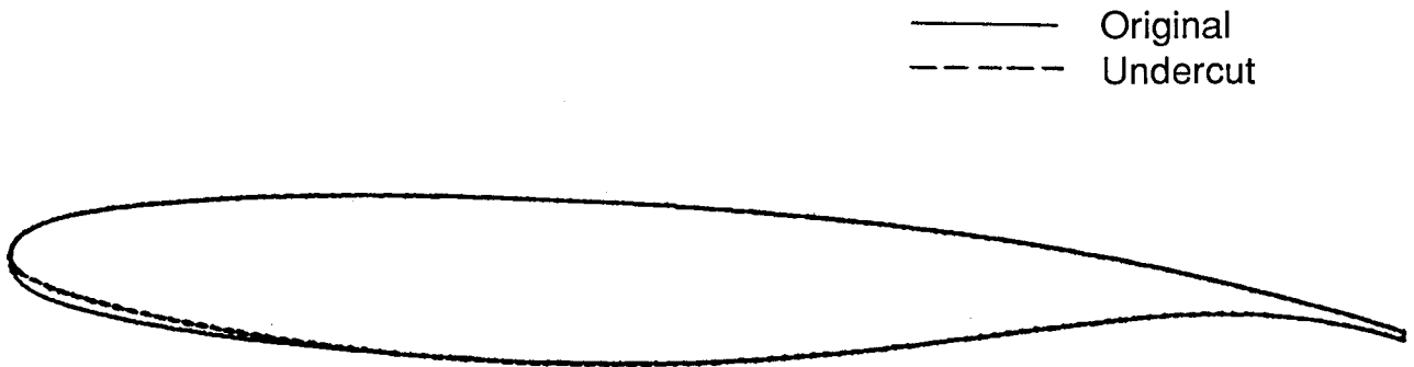
Figure 31. Sketches of 12-percent-thick supercritical airfoil with and without forward lower-surface undercutting.
