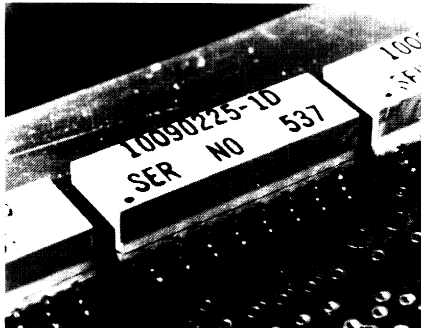
Fig. 15. JPL DIP interface transformer package
