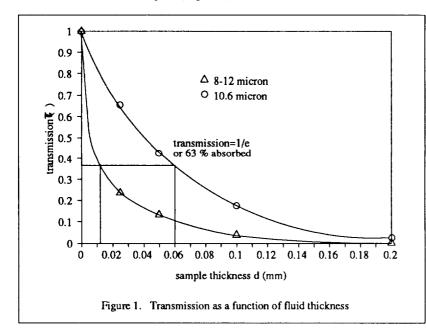
incoming radiation is found to be 0.200 mm and 0.256 mm for the  $8-12\mu$  region and 10.6 wavelength respecively. μ Therefore, it is concluded that the "surface" the imager "sees" is 0.200 mm thick. The fact that the CO<sub>2</sub> laser radiation penetrates deeper than this is advantageous. If the situation were reversed, the temperature indicated by the imager would an average over a region he where a much larger temp-
