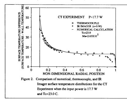
heater of 17.7 W. Plotted in the figure is the surface temperature difference between the surface oil the test chamber wall against nondimensional position, measured radial with the target emissivity set to 0.90. The agreement among the three techniques for this case is  $\pm 5\%$  of the overall  $\Delta T$ excluding the near wall regions. The errors in the wall regions are  $\pm 10\%$  of the  $\Delta T$  and are caused. predominantly, by the
