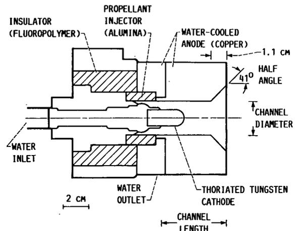
FIGURE 2. - MPD THRUSTER (D) WITH FLARED ANODE.
