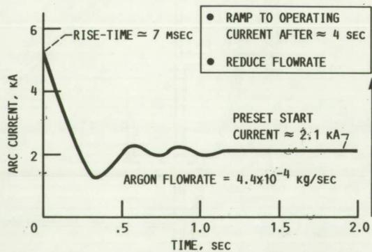
FIGURE 11. - TYPICAL ARC-START AFTER BREAKDOWN WITH IGNITOR SUPPLY.
