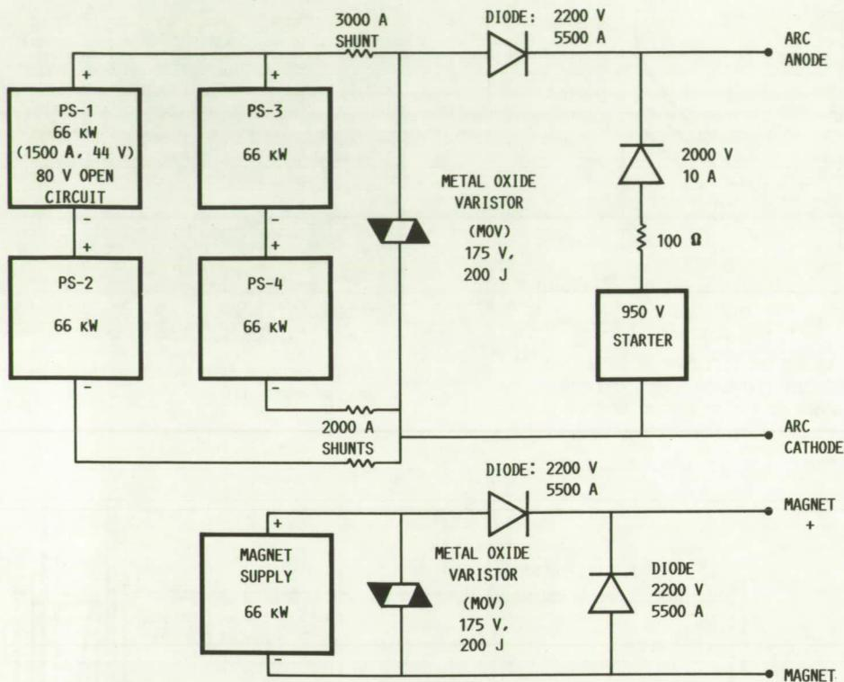
FIGURE 9. - POWER SYSTEM SCHEMATIC. (INPUT POWER: 3Φ, 460 V; POWER CABLES: (FOUR EACH) 777 MCM CABLES FOR 3000 A.)
