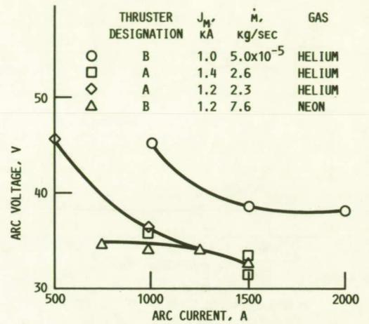
FIGURE 13. - MPD THRUSTER DISCHARGE CHARACTERISTICS WITH HELIUM AND NEON.
