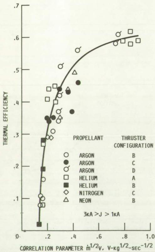
FIGURE 18. - THERMAL EFFICIENCY CORRELATION PARAMETER.
