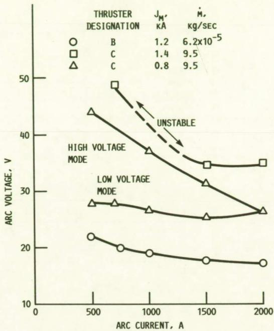
FIGURE 12. - MPD THRUSTER DISCHARGE CHARACTERISTICS WITH ARGON.
