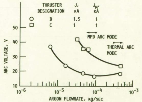
FIGURE 14. - SENSITIVITY OF ARC VOLTAGE TO ARGON MASS FLOWRATE.
