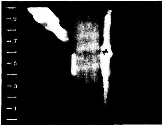
FIGURE 13. INFRARED IMAGE OF TEST MODEL SUPPLIED WITH 150°F AIR.
