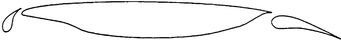
(c) 10-percent leading-edge flap configuration.
