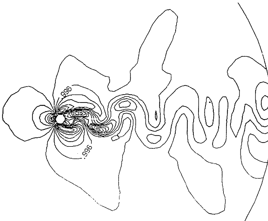
Figure 5.1b: Temperature contour plot of the spectral scheme SP1 at Time = 803.255 .
