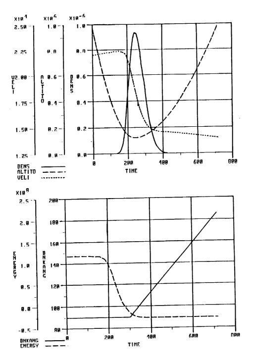
Figure 1. Baseline trajectory showing Martian aerocapture using two bank angle commands and flying through a deterministic atmosphere.
