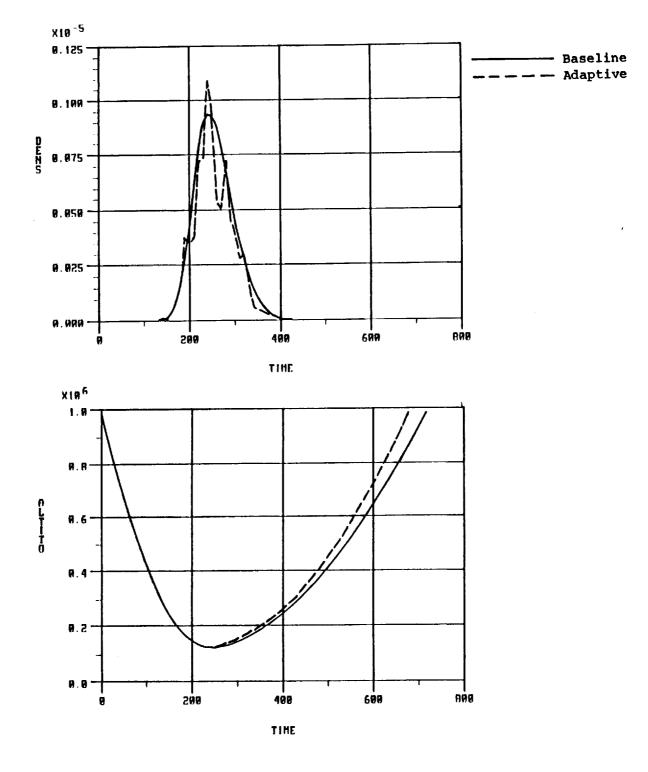
Figure 5. State and atmosphere time histories for a Martian aerocapture using adaptive guidance 1, with a reduced gain of  $1 \times 10^{-4}$ , flying through a random atmosphere with maximum density variations of 50 percent and for the baseline trajectory.
