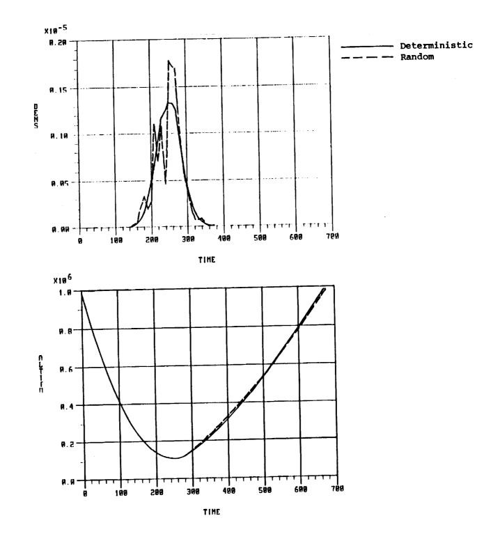
Figure 7. State and atmosphere time histories for a Martian aerocapture using adaptive guidance 2, flying through a random atmosphere with maximum density variations of 86 percent and for a deterministic atmosphere.
