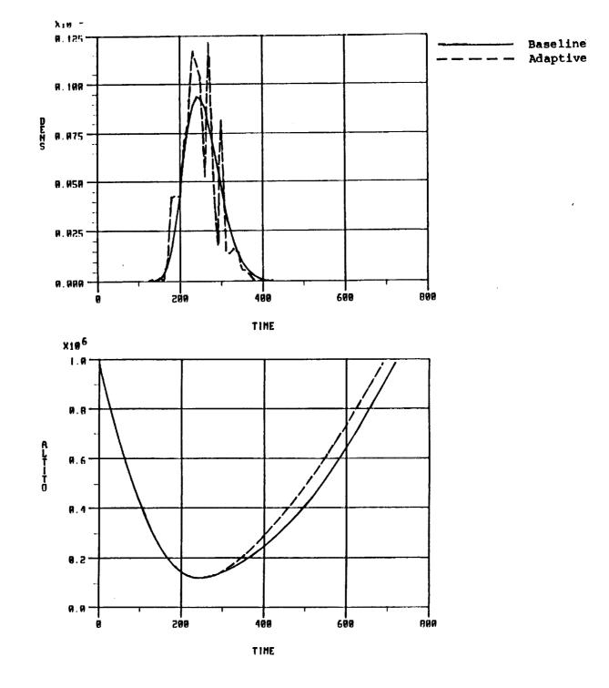
Figure 3. State and atmosphere time histories for a Martian aerocapture using adaptive guidance 1, with a reduced gain of 1x10<sup>-4</sup>, flying through a random atmosphere with maximum density variations of 86 percent and for the baseline trajectory.
