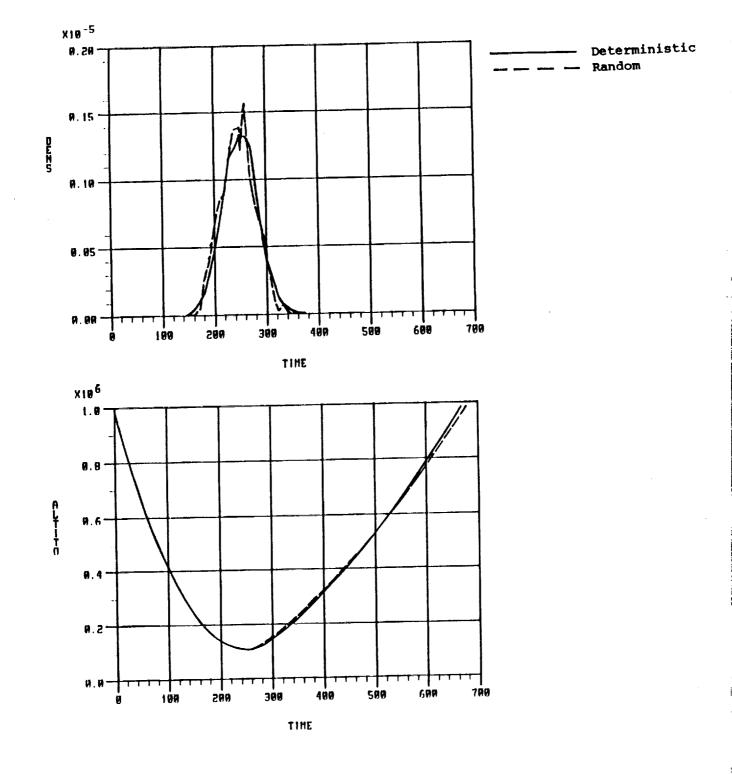
Figure 6. State and atmosphere time histories for a Martian aerocapture using adaptive guidance 2, flying through a random atmosphere with maximum density variations of 50 percent and for a deterministic atmosphere.
