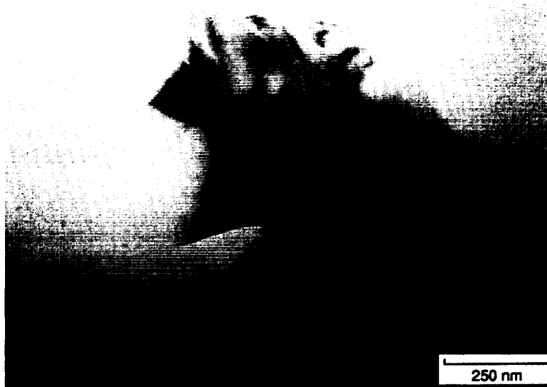
(c) Brittle fractured wear debris particle. Note no dislocations or evidence of plastic behavior detected.
