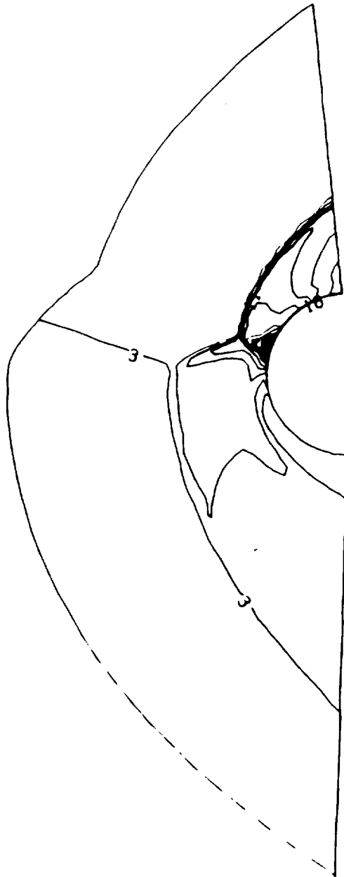
Fig. 5.33 Density contours for the cowl forebody, M_\infty = 8.03 .
