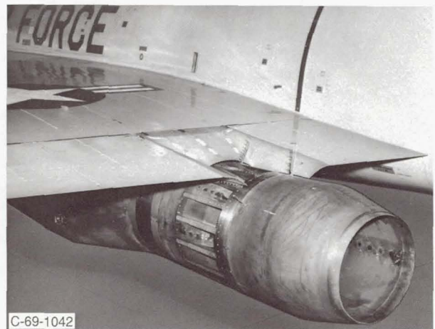
Figure 5-25.—Auxiliary-inlet ejector nozzle installation and elevon trough.
