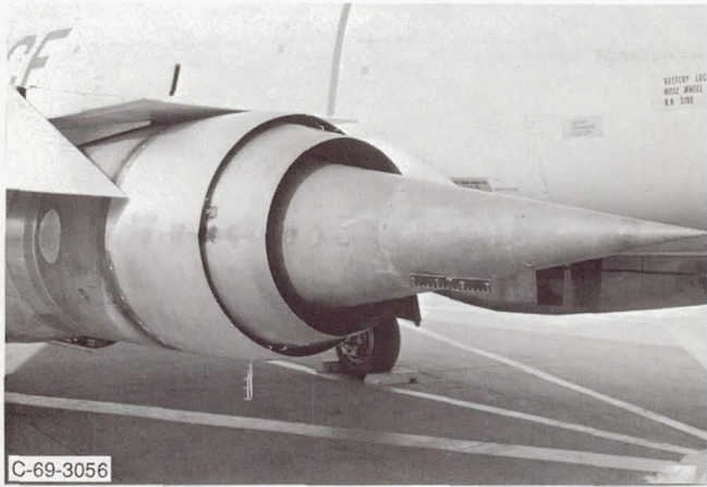
Figure 5-28.—Low-angle plug nozzle installation.
