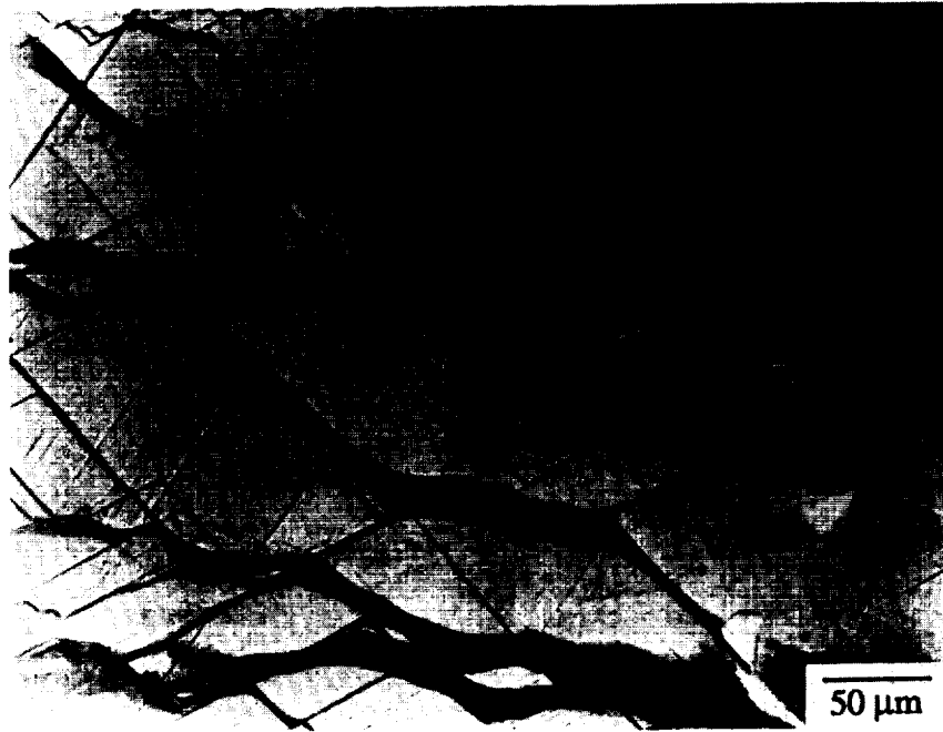
Figure 4.24 Compression slip bands at \epsilon_p = 1.3\% .
