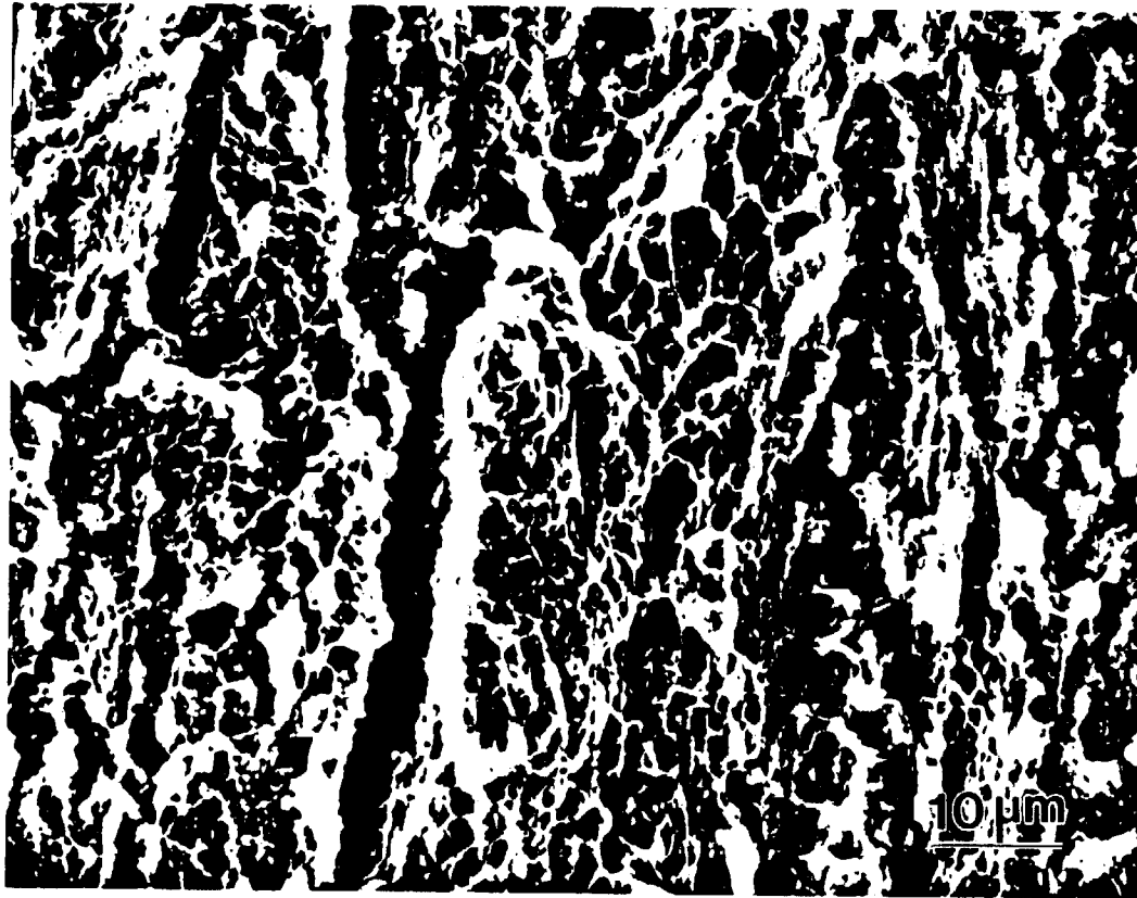
Creep crack growth fracture surface of FVS0812 (175 °C)
