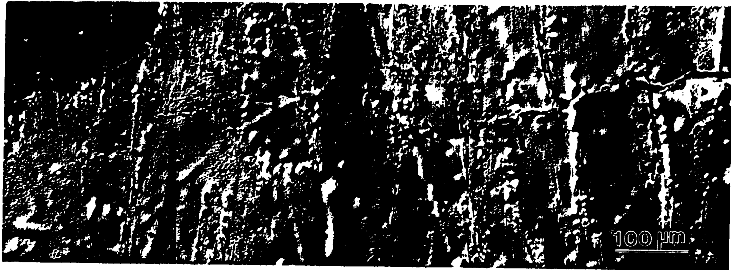
Nomarski contrast micrograph of the crack path profile of FVS0812 Al alloy after creep crack growth tested at 316 °C
