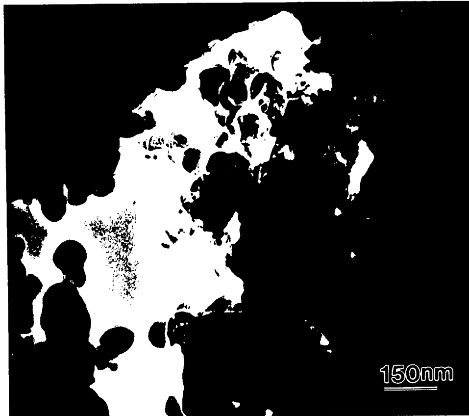
TEM micrograph of the crack tip of FVS0812 Al alloy after CCG tested at 316 °C
