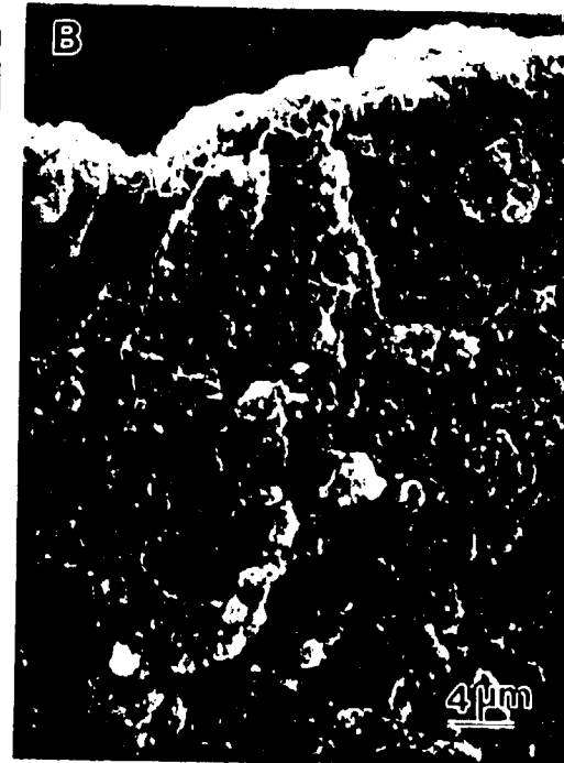
Side views of CCG fracture surface of FVS0812 (175 °C) a) dimple fracture region b) delamination region
