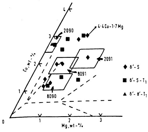
Precipitate phases reported in quarternary Al-Cu-Mg alloys containing 2-3 wt-%Li in material aged at 190°C; where original source quotes composition range, centre of that range has been used as composition shown here; composition ranges of internationally designated Al-Li-Cu-Mg alloys and precipitate phase fields of ternary Al-Cu-Mg system at 190°C are also shown
