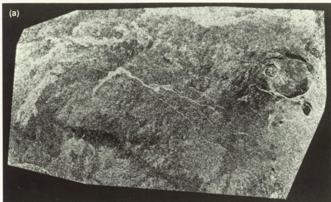
Figure 24. SIR-B images of the central parts of the swaths over Hawaii, including the Kau Desert and Kilauea Crater: (a) image obtained at 28-deg look angle; (b) image at 48-deg look angle. Note differences in the response of vegetated areas to the right of Kilauea Crater. These images have not been corrected for scale-factor differences.
