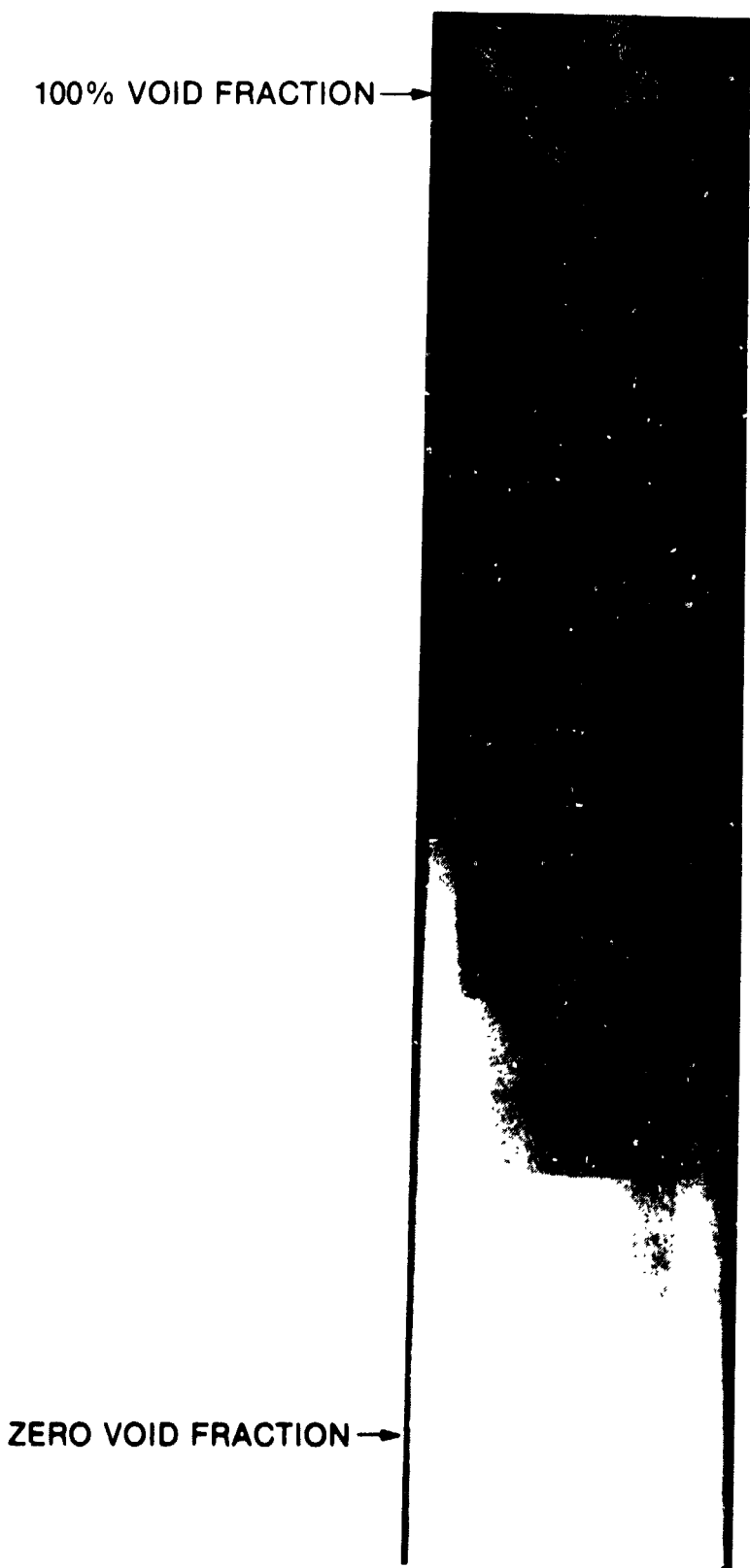
Figure 4. X-Ray Photo Negative of the Stepwedge Calibration
